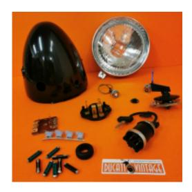
Complete black drop shape headlight - but electronic type - Ducati Scrambler type 1st series with original electronic ignition engine, original model of transition between 1st and 2nd series
