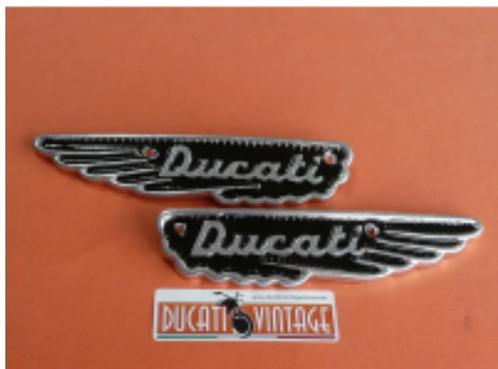
Pair of wings for Ducati Scrambler tank painted realized in forged aluminium identical to the originals in every detail. is a product Made in Italy
