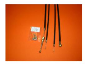
Kit cables: front brake-starter-throttle-clutch for Ducati Scrambler 1st series
