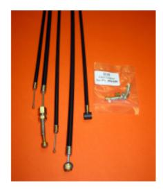
Kit cables:front brake,starter,throttle,clutch,decompressor lifter Du Ducati Scrambler 1° s.
