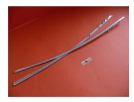
Pair original aluminium profiles with screws to fix the seat Ducati RT cover
